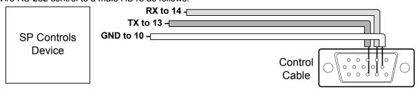
Connect male HD15 to 3M port labeled *CONTROL*. Serial Adapters (for NRC only): B and C
