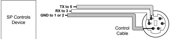
Connect male mini-DIN to projector port labeled RS-232. Serial Adapters (for NRC only): n/a
