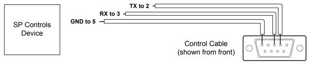
Connect female DB9 to projector port labeled *RS-232*. *Serial Adapters* (for NRC only): None
