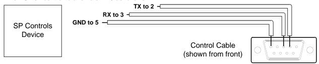
Connect female DB9 to projector port labeled *SERIAL*. Serial Adapters (for NRC only): None
