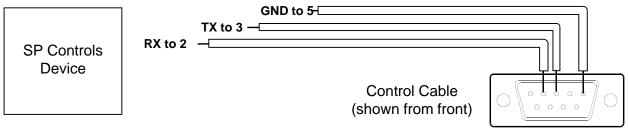
Connect male DB9 to Mitsubishi RS-232 mini-DIN adapter cable. Connect adapter cable to the projector port labeled *RS-232C*.
