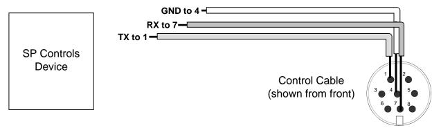
Connect the male mini-DIN to the projector port labeled RS-232C.
