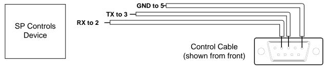
Connect male DB9 to custom NEC RS-232 adapter cable (included with projector), and connect adapter to the projector port labeled *PC Control*.
