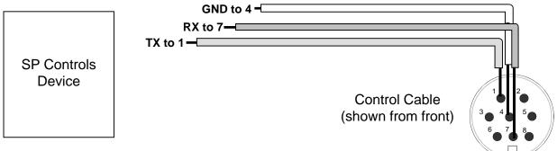
Connect 8-pin mini-DIN to projector port labeled *PC CONTROL*. *Serial Adapters* (for NRC only): N/A
