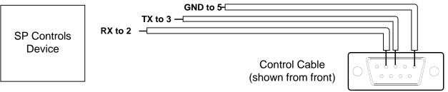
Connect male DB9 to projector port labeled *Serial. Serial Adapters* (for NRC only): A and B
